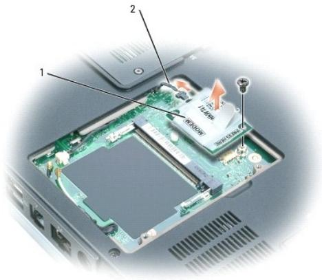
10. Turn the computer over and disconnect the modem cable from the system board connector.
