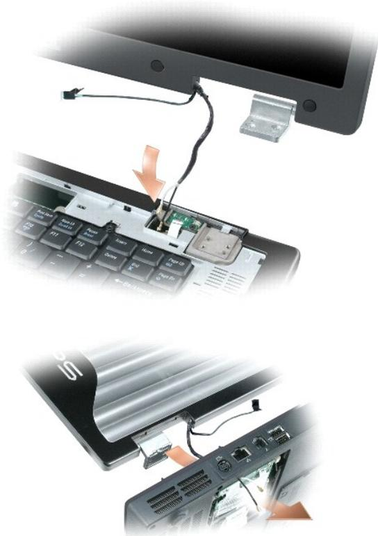
4. Connect the LED cable to the system board.
