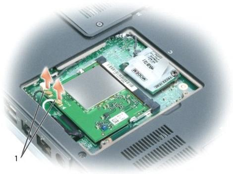
➡ **NOTICE:** To prevent damage to the Mini PCI card connector, do not use tools to spread the securing clips that secure the card.
