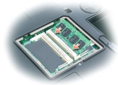
2. Replace the memory cover and tighten the captive screws.
