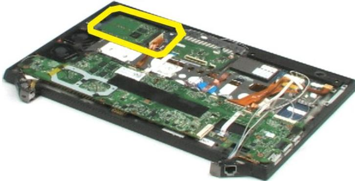
5. Disconnect the hard-drive cable from the connector on the system board.
