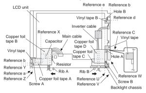
Make sure to align the edges of the inverter PWB with those of insulating sheet before attaching the Put it over and attach with
