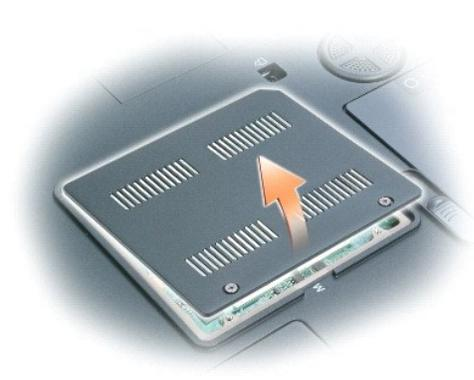
**➡ NOTICE:** To prevent damage to the memory module connector, do not use tools to spread the securing clips that secure the memory module.
