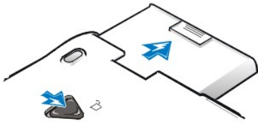
Figure 2. Installing a Battery
