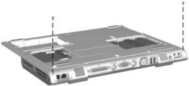
Figure 5-38. Removing the Top Cover Screws
