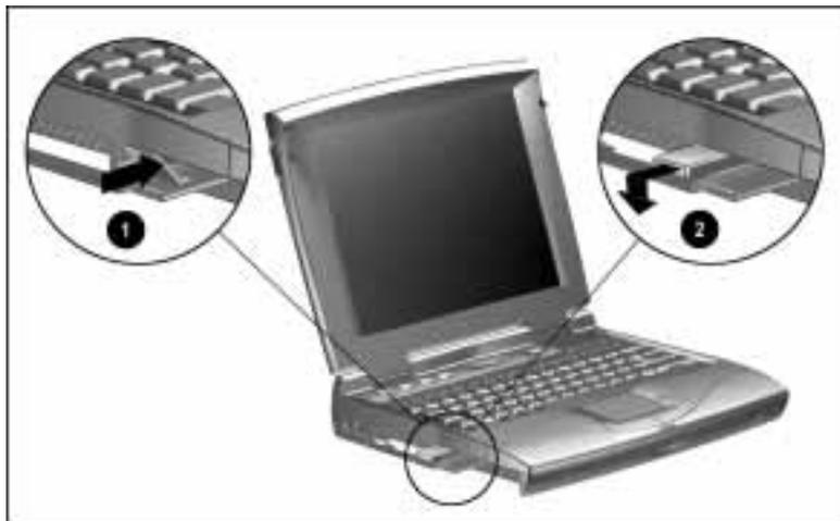
Figure 1-1. New Battery Spacer Door
