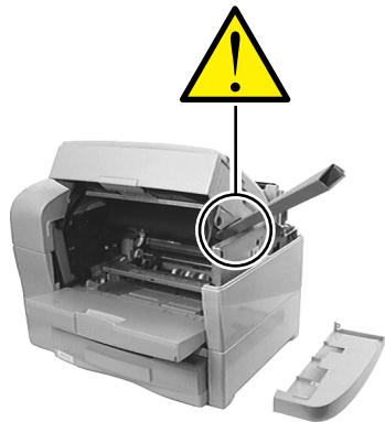
Temporary Support For Top Cover
