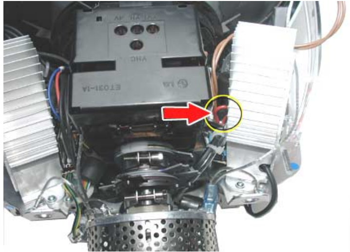
Voltage Jumper Location
